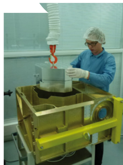
A complete dummy of the MATISSE Cold Optics Box was created as a verification model for the thermal properties. In the picture you see the gold colored backbone of about 70 kg, cut from a solid block of aluminum of 600 kg. It has been the largest part ever milled on ASTRON's big milling machine. In September 2012, the thermal dummy COB was shipped to MPIA Heidelberg, exactly on schedule. Credits: NOVA optical infrared group at ASTRON.
