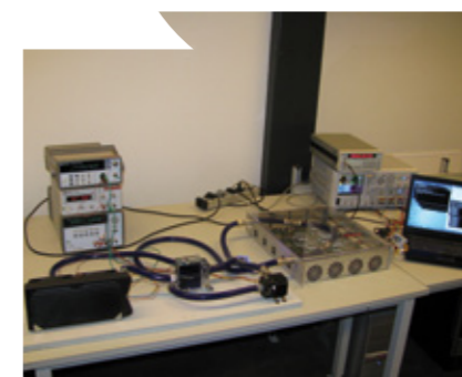
Set-up demonstrating liquid cooling of a UniBoard processing board.
