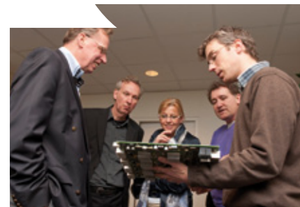
Instrument engineer Gijs Schoonderbeek shows visitors of VNO-NCW Noord the Uniboard, compact hardware that can process as much as 120 GB of (telescope) data per second.
