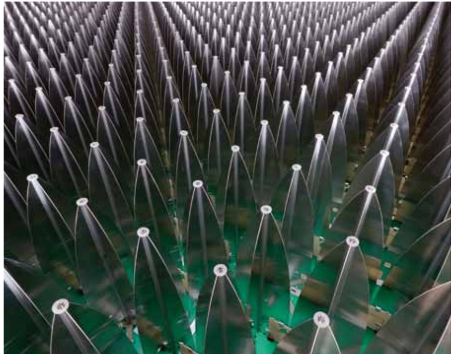
Array of small antennas in the EMBRACE demonstrator to replace moving dishes.
