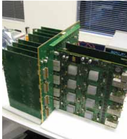
APERTIF beamformer subrack.
