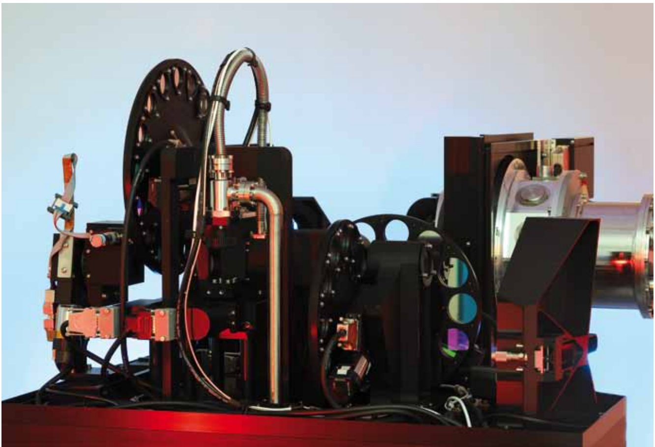
The ZIMPOL instrument without cover, located in the cleanroom at ASTRON for a last overhaul before shipment to Grenoble. Light will enter the instrument from the left, provided by the general optics of SPHERE. Clearly visible are the wheels for filter and polarization components. In the middle a vacuum tube is leading to the FLC, the hart of the instrument. On the right hand side, the cryostat is visible. The two detector CCDs are located in the cryostat.
