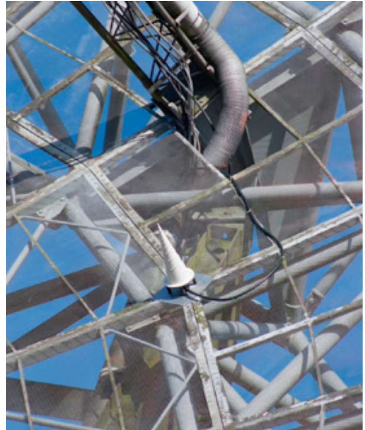
Calibration antenna for Galileo mounted in one of the WSRT dishes
