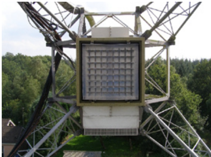
Focal plane arrays in the focus of one of the Westerbork dishes
