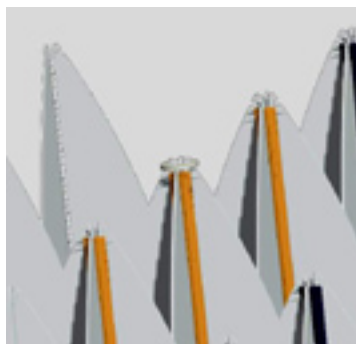
The devil is in the details... Plastic rings added on top of the Vivaldi elements to prevent occasional minor displacements during transport.
