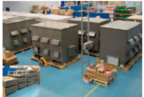
LOFAR cabinets in storage at Excel Assemblies in Emmen. The digital and analogue printed circuit boards and other equipment are placed inside these cabinets before they are shipped to the fields. The small inset image in the lower left shows the PVC pipes that are used in the Low Band Antenna.
