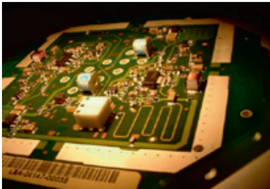
The LBA-LNA is the Low Noise Amplifier of the LOFAR Low Band Antenna. The picture shows a circuit board with two such amplifiers, one for each of the two polarizations of the incoming radio signals. The LNA has been optimized to work in the low frequency band from 30MHz to 80MHz. The four antenna wires will be soldered to the printed circuit board, forming two highly sensitive dipole antennas. Then the electronics will be sealed in, protected against wind, rain and sunshine (photograph Henri Meulman).
