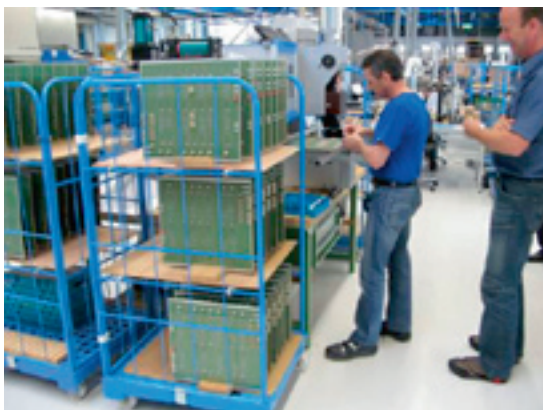
Production of the LOFAR Backplanes which will connect the analogue processing on one side (in particular the receivers) and the digital processing boards on the other side (photograph: Menno Norden, Gijs Schoonderbeek).
