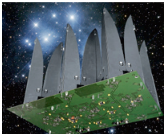
Not an artist impression, but the celebration picture of the first EMBRACE receiver board. These so-called Hex-boards, placed together in groups of six, each contain 24 Vivaldi elements (dual-pol), low noise amplifiers and analogue beamformer chips (developed in France) and switchable True-time-delay lines. (Photograph: Jürgen Morawietz, ASTRON. background image: Albert van Duin, ASTRON).
