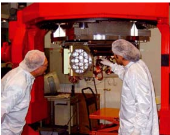
The integrated cold optical box mounted on the VLT simulator at ASTRON
