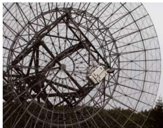
The Digistif system in the focus one of the WSRT dishes.
