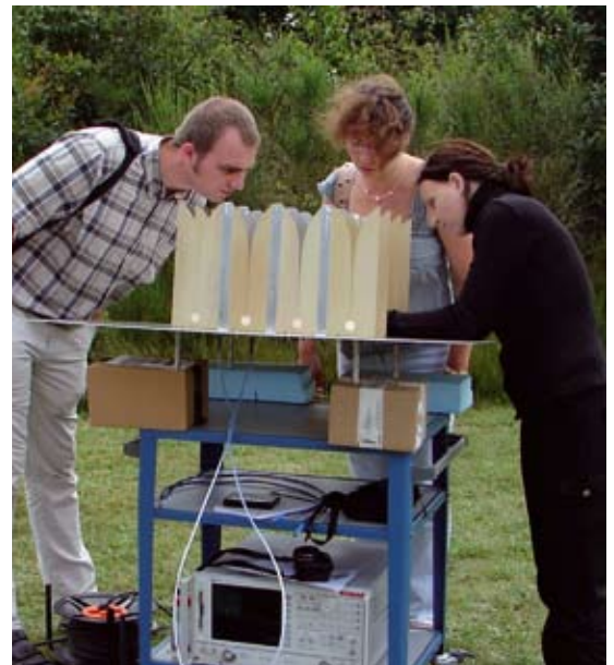
Ms. Redkina performing the measurements of the scattering parameters of the 16-Vivaldi element array
