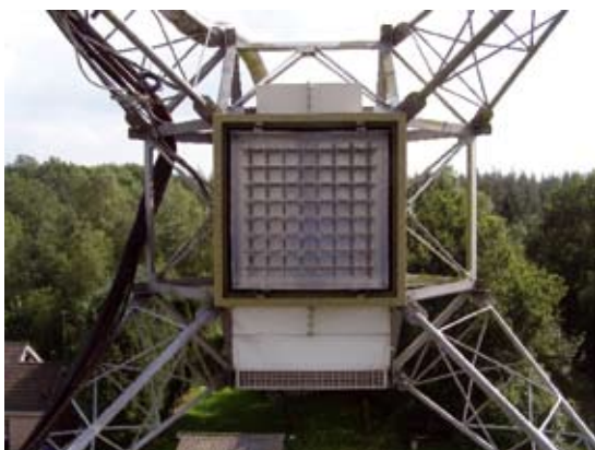
Digestif focal-plane array on one of the dishes of the Westerbork telescope
