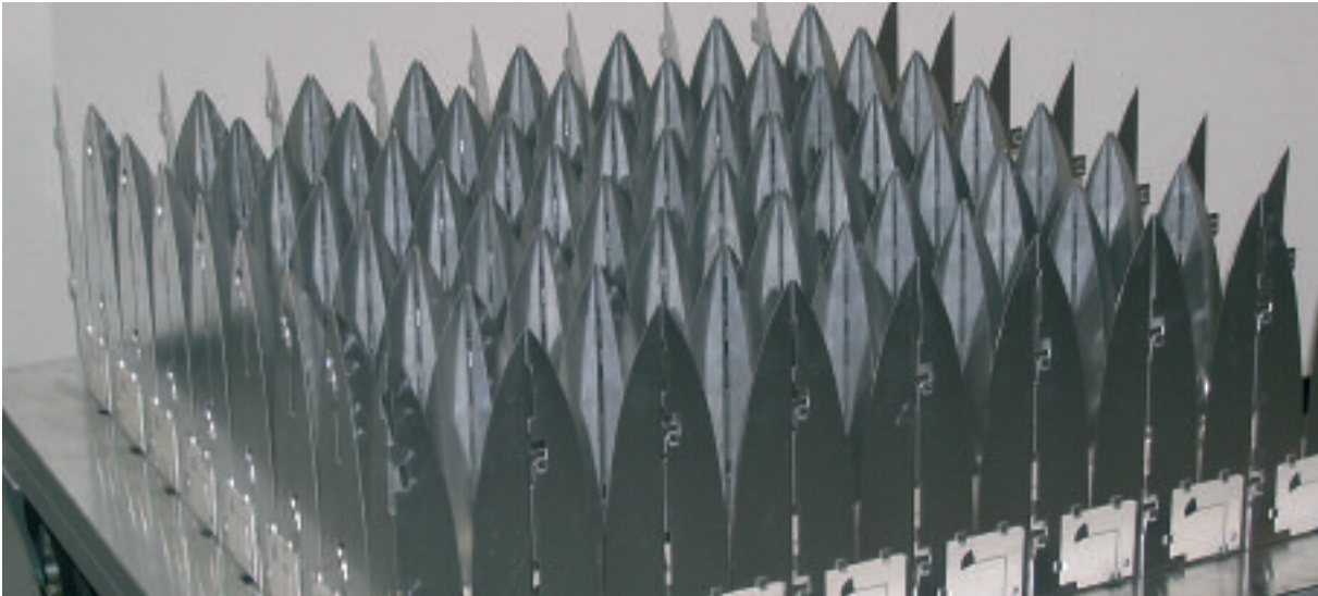
The first EMBRACE tile, primarily used to verify the antenna patterns.
