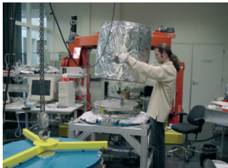
The test cryostat, designed for qualification tests of MIRI (Mid Infrared Instrument for the James Webb Space Telescope) is integrated for the first cold run. The picture shows ASTRON test and support engineer Eddy Elswijk mounting the cold screen (50K).
