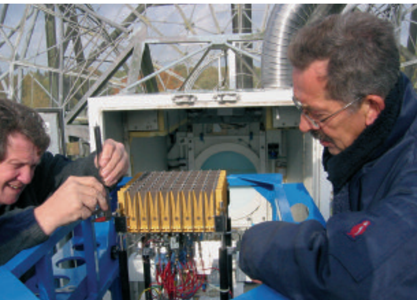
ASTRON engineers Harm-Jan Stiepel and Kees Brouwer are mounting the FPA feed on one of the WSRT telescopes.
