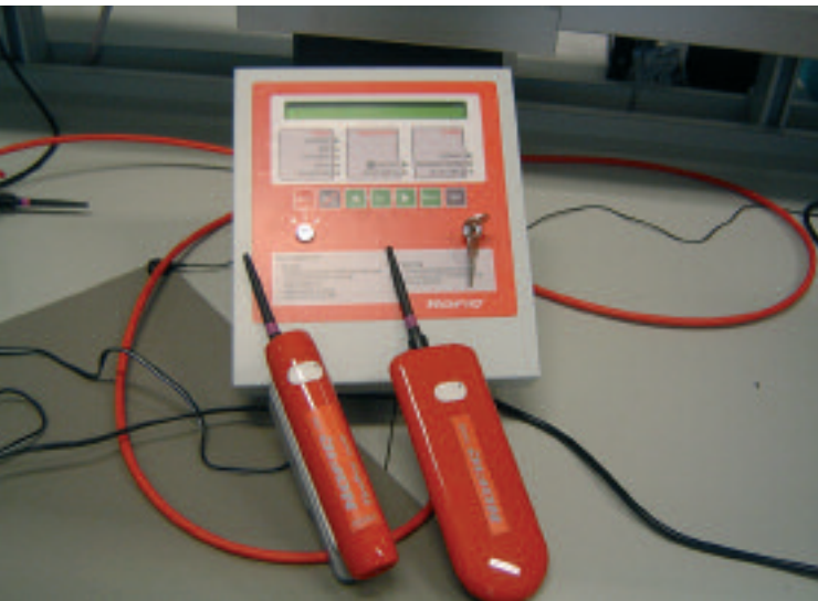
NOFIQ is an early-stage fire detection and source extinguishing system which, when sensing the early signs of a fire near fire extinguishing units, sends a alerting signal by a 2.4 GHz wireless connection network to the main control unit. Then the relevant extinguishing units will release autonomous a gas (harmless to electronics and humans) to extinguish the fire. (copyright Astrotec Holding B.V.)
