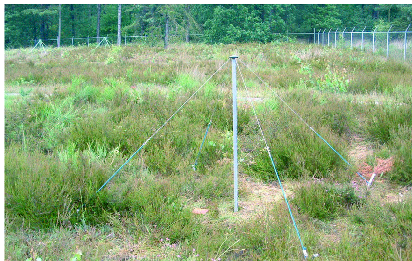
Prototype of the LOFAR LBA antenna.
