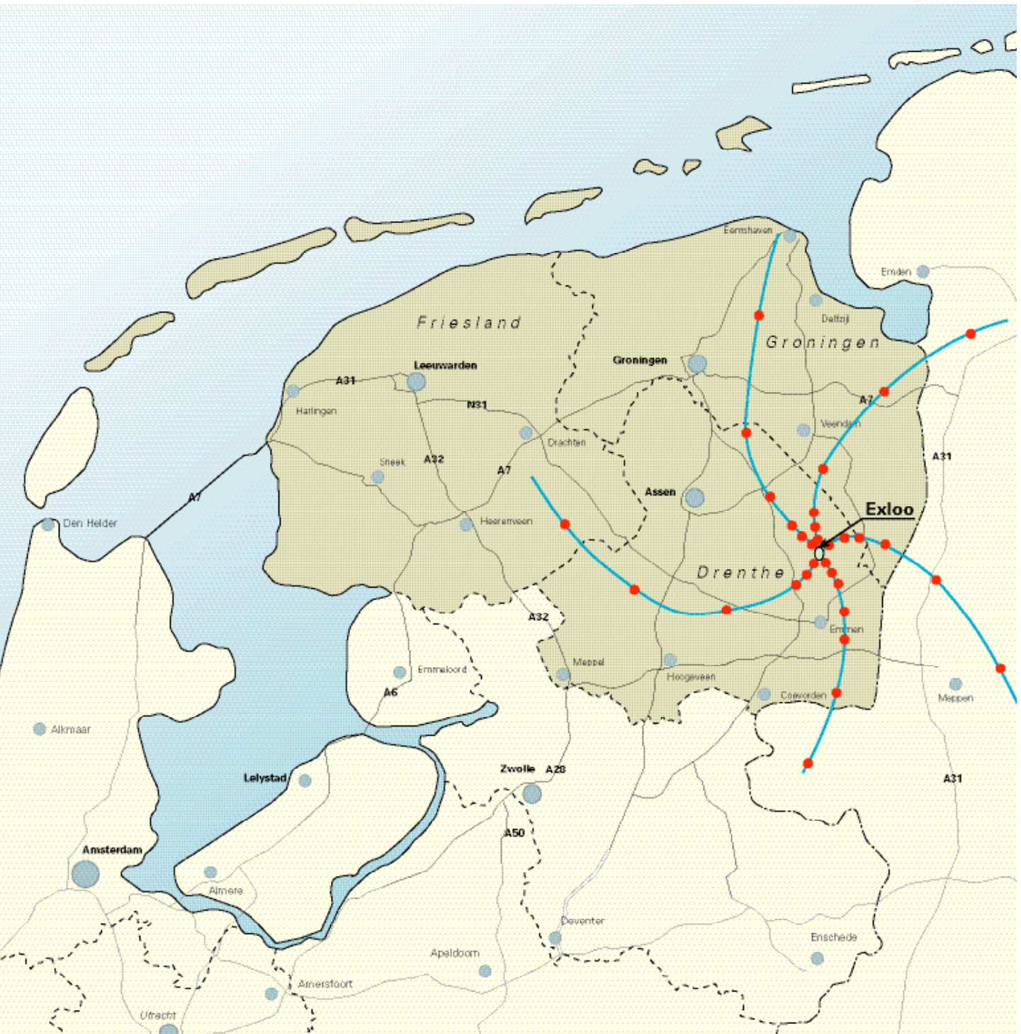
First phase of the LOFAR sensor network. Each red dot represents a (sensor) station.
