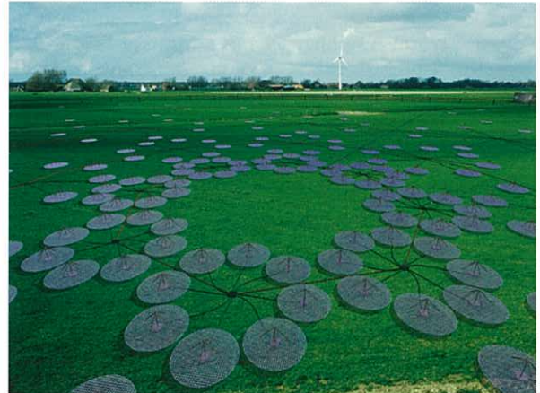
Figure 2.16 Artist's impression of a LOFAR Station in a generic landscape (above), and below an illustration of the way in which the receiving elements are combined to form beams on the sky.
