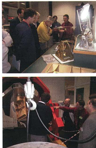
Figure 7.1 A group of visitors being shown round ASTRON’s facilities. These images show a tour of the VISIR integration room, with (top) a description of the mirrors being produced and (bottom) a full scale dummy of the mechanical interface to a unit VLT telescope.
