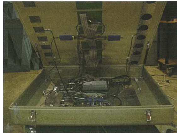
Figure 2.2 The first THEA tile being assembled in the Lab. The top image shows the 64 single polarized elements, the lower image the tile's electronics in a shielded area below the elements.
